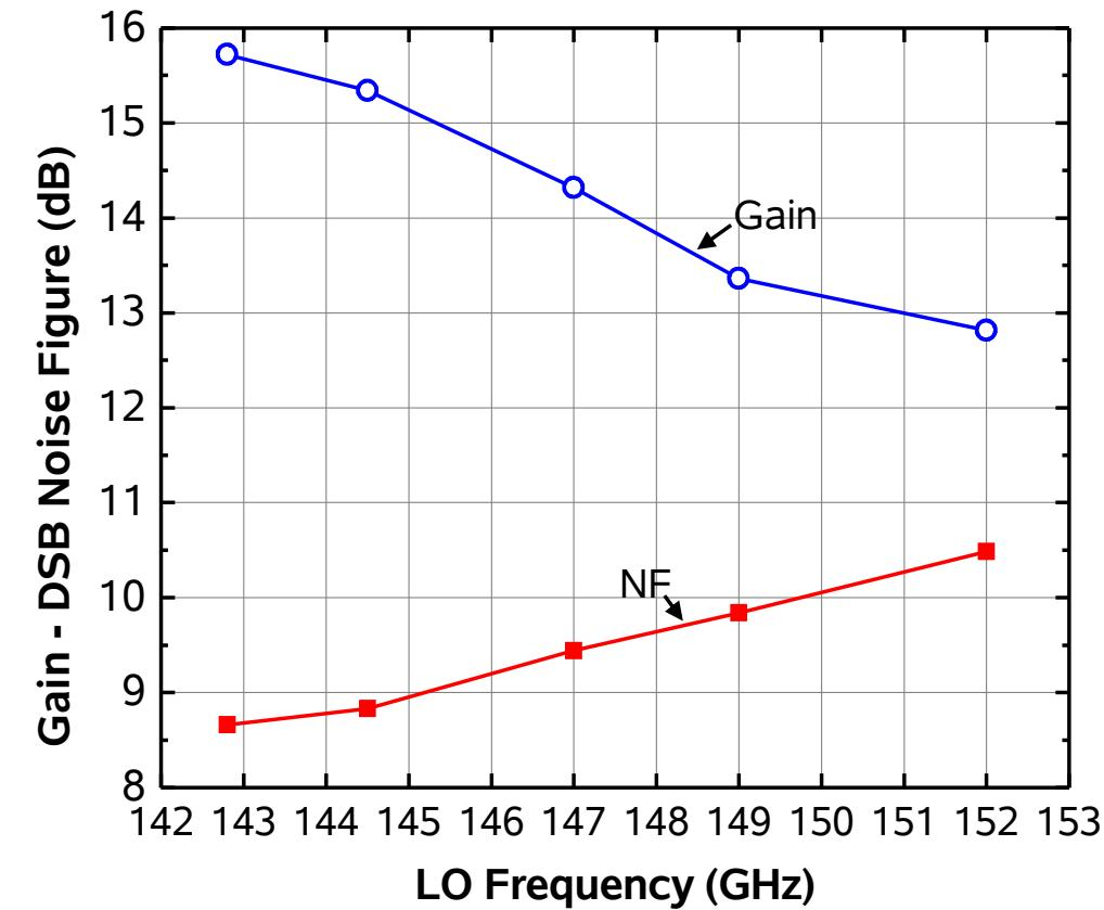
**13-15 dB gain, 23 dB of gain control in LNA**
