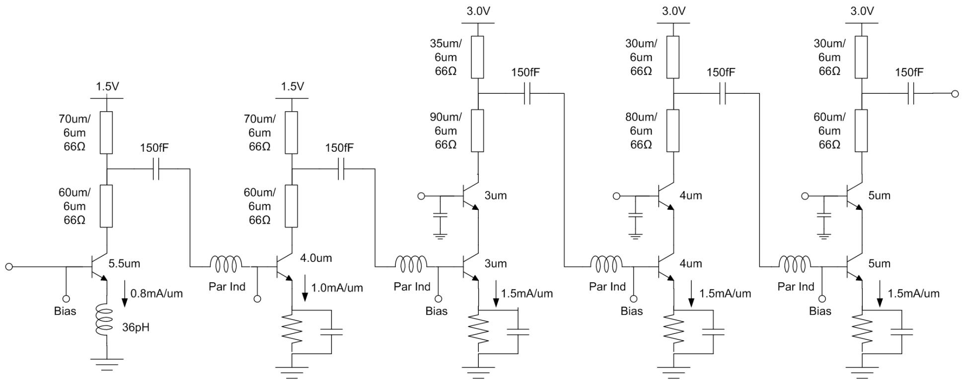
$P_D = 67 \text{ mW}$ , Gain= 20 dB, NF < 12 dB.
