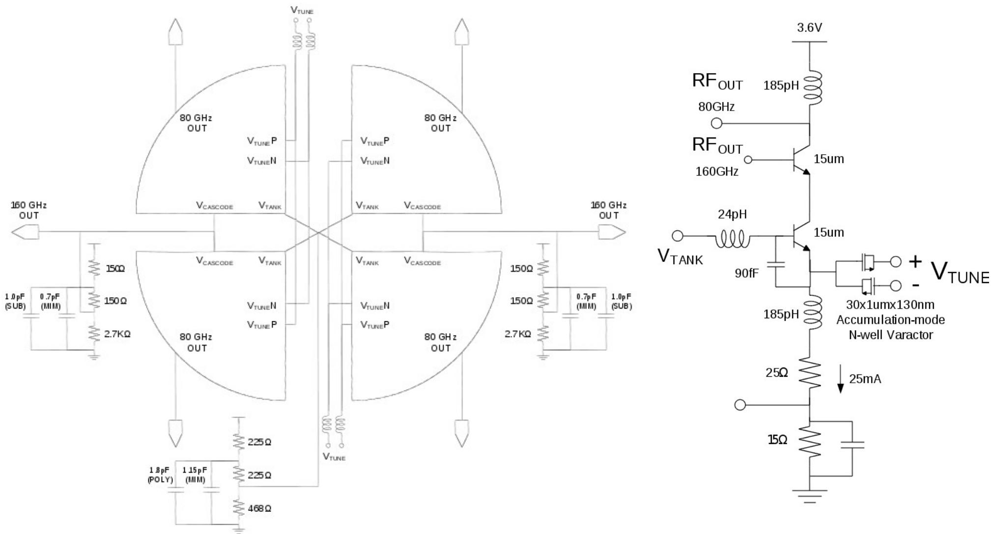
$$P_{DC} = 360 \text{ mW}, P_{OUT} = -10 \text{ dBm}, PN = -82 \text{ dBc/Hz at } 1 \text{ MHz offset}$$
