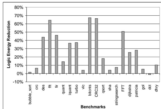
Fig. 13. Energy reduction of subsetting on 3-stage pipeline.
