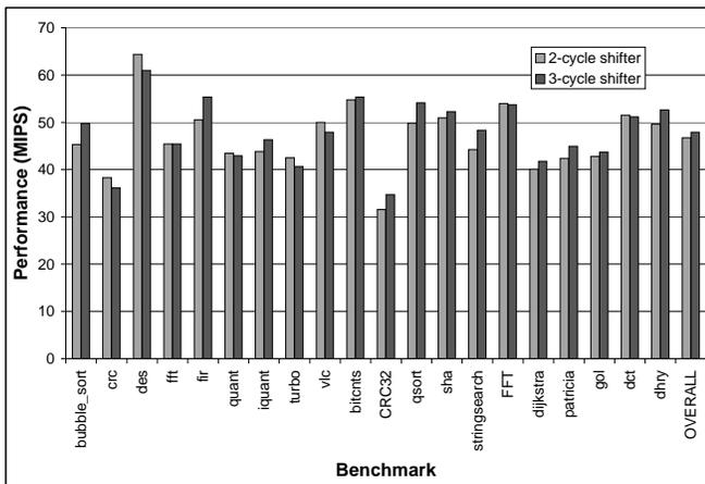
Fig. 8. The performance trade-off in implementing unpipelined multi-cycle paths on a processor across the benchmark set.
