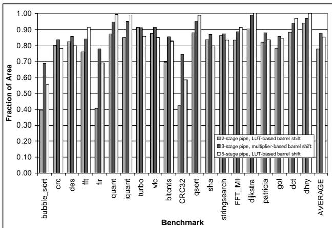
Fig. 11. The impact on area of ISA subsetting on three architectures.
