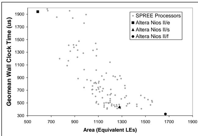
Fig. 2. Comparison of our generated designs vs the three Altera Nios II variations.
