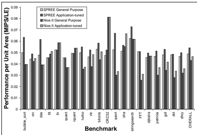
Fig. 9. Performance-per-area for each benchmark for SPREE (i) best-on-average (*general-purpose*) processor and (ii) best per benchmark (*application-tuned*) processor as well as for Nios II (iii) general purpose and (iv) application tuned.
