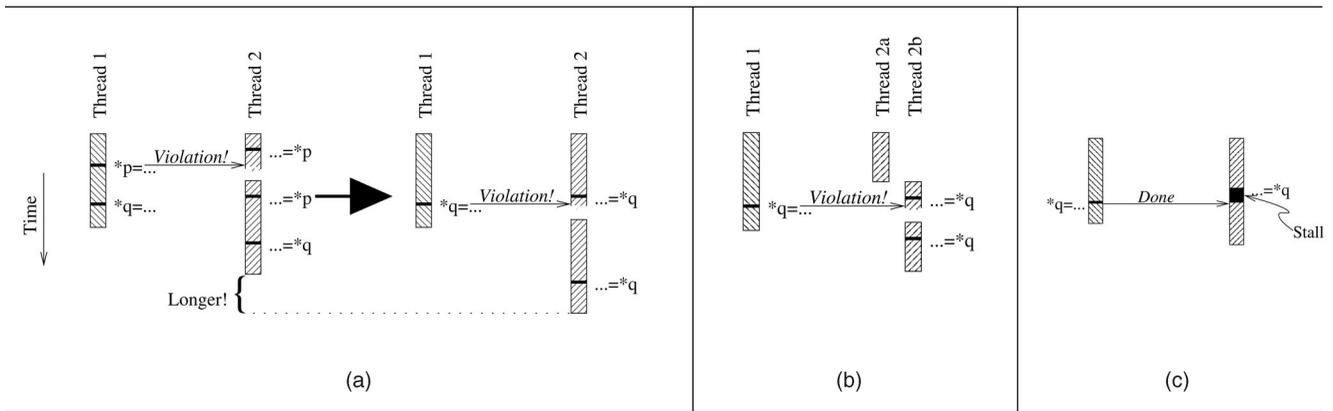
Fig. 1. The use of subthreads enables a performance tuning process, where eliminating data dependences improves performance. (a) Eliminating the dependence through  $*p$  can potentially *hurt* performance with an all-or-nothing TLS execution. (b) Execution with subthreads. (c) Idealized parallel execution.
