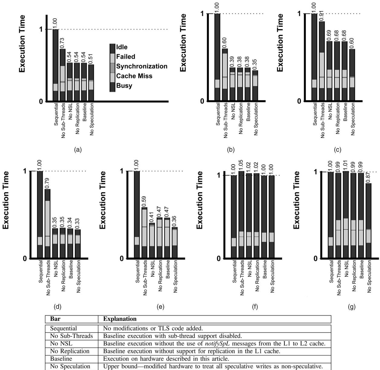
Fig. 5. Performance of optimized benchmarks on four CPUs run sequentially, without subthread support, without the *notifySpL* message, without replication in the L1 cache, with full support, and with an upper bound where there is no speculation. (a) NEW ORDER. (b) NEW ORDER 150. (c) DELIVERY. (d) DELIVERY OUTER. (e) STOCK LEVEL. (f) PAYMENT. (g) ORDER STATUS.
