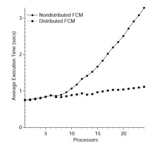
Fig. 12. Graph of distributed FCM and nondistributed FCM performance. One instance of grep is executed on each processor. Each grep searches a common 111MB file for a common nonmatching search pattern. The graph shows the average grep completion time.
