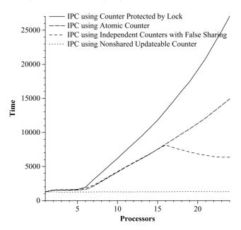
Fig. 1. K42 microbenchmark measuring cycles required for parallel client-server IPC requests to update a counter. Locks, shared data access, and falsely shared cache lines all increase round-trip times significantly even though the shared data access constitutes less than one tenth of one percent of the overhead in the uncontended case.
