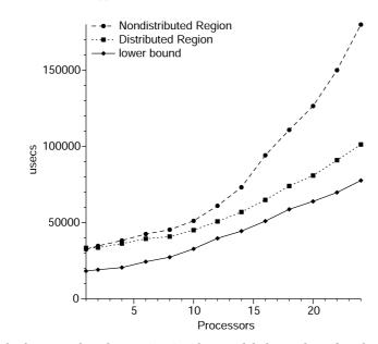
Fig. 9. Graph of average thread execution time for a modified memclone. One thread is executed per processor. Each thread touches 2500 independent pages of a **single** large common memory allocation. Each page touch results in a zero-fill page fault in the OS. The graph plots the performance when using a nondistributed versus a distributed Region object to back the single common memory allocation. The lower bound performance for concurrent zero-filling is included for reference.
