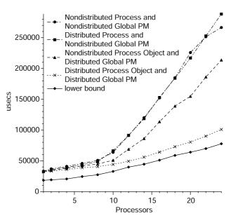
Fig. 8. Similar to Figure 6. Graph of average thread execution time for memclone running on K42.
