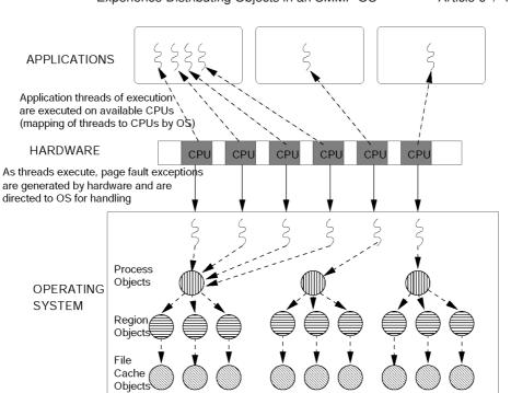
Fig. 2. An illustration of the K42 runtime structure used to handle in-core page faults.
