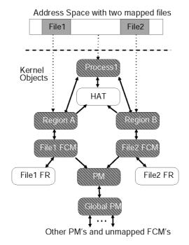
Fig. 4. VMM object network representing an address space with two mapped files.
