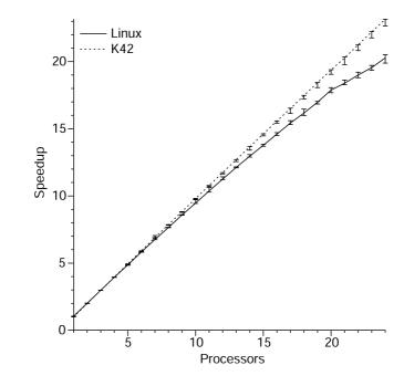
Fig. 16. Speedup of *p* independent instances of Make normalized to K42 uniprocessor result.
