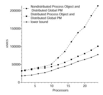
Fig. 6. Graph of average thread execution time for memclone running on K42. One thread is executed per processor. Each thread touches 2500 pages of an independent memory allocation. Each page touch results in a zero-fill page fault in the OS. The performance of using non-distributed and distributed Process objects is shown. In both cases the distributed Global PM object is used. The lower-bound for concurrent zero-filling of memory on the S85 is included for reference.
