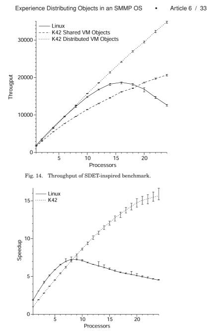
Fig. 15. Speedup of p independent instances of Postmark normalized to K42 uniprocessor result.
