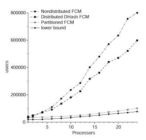
Fig. 13. Similar to Figure 9. Graph of average thread execution time for a modified memclone, as described in the text, running on K42. The graph plots the performance of using a nondistributed FCM versus a distributed FCM, using DHash versus a partitioned FCM, to back the single common memory allocation.
