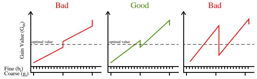
• the fine control DAC range is a function of the coarse control bits
