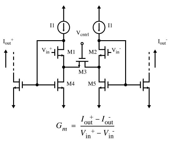
•  $G_m$  is proportional to triode-transistor, M3, conductance
