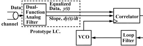
Fig. 2. Proposed MMSE TR scheme.
