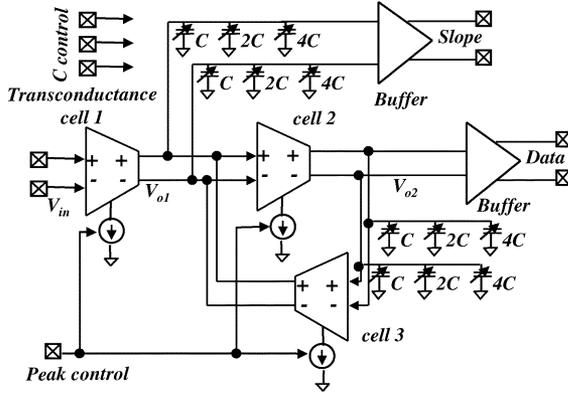
Fig. 4. Dual-function analog filter topology.
