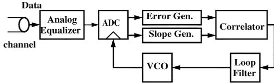
Fig. 1. Conventional MMSE TR scheme.
