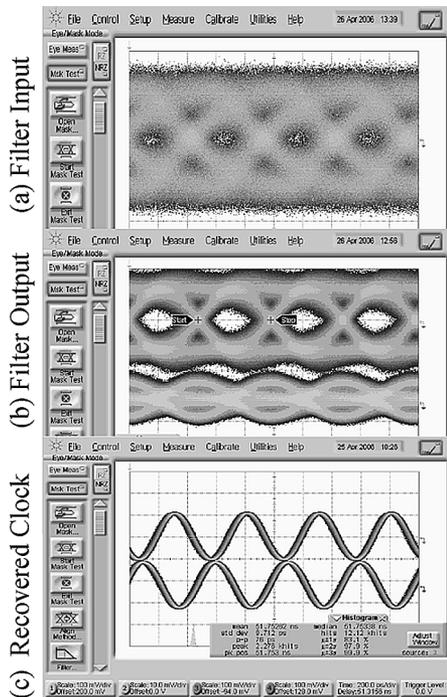
Fig. 11. Eye diagrams at different points of the TR loop. (a) Channel output/filter input at 2-Gb/s (Vertical scale = 25 mv/div; Horizontal scale = 200 ps/div), (b) Equalized data (top) and slope (bottom) outputs of dual-function analog filter at 2-Gb/s (Vertical scale = 25 mv/div; Horizontal scale = 200 ps/div), and (c) Recovered clock at 2-GHz (Vertical scale = 100 mv/div; Horizontal scale = 200 ps/div).
