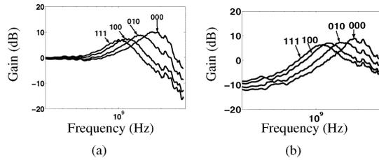
Fig. 6. Measured frequency response for four different digital control word inputs to the binary weighted capacitor bank of the dual-function analog filter. (a) Data path. (b) Slope path.
