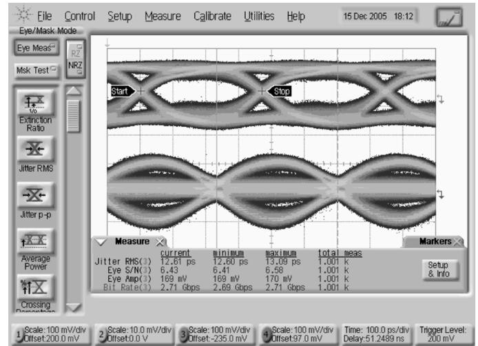
Fig. 7. Data (top eye) and slope (bottom eye) outputs of dual-function analog filter at 2.7-Gb/s (Vertical scale = 100 mV/div; Horizontal scale = 200 ps/div).
