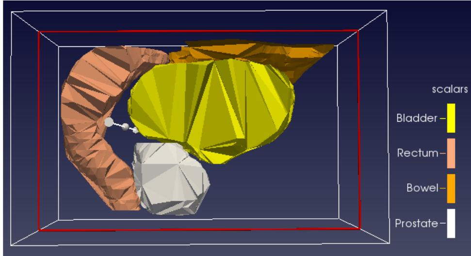
Figure 2. Cut showing the poor-quality, long, thin tetrahedra (108k elements total) before refinement. Tetras composing the surrounding tissue (not shown to avoid clutter) are particularly large. Long tetrahedra cause excess fluence averaging along their long axis, which hurts result quality.
