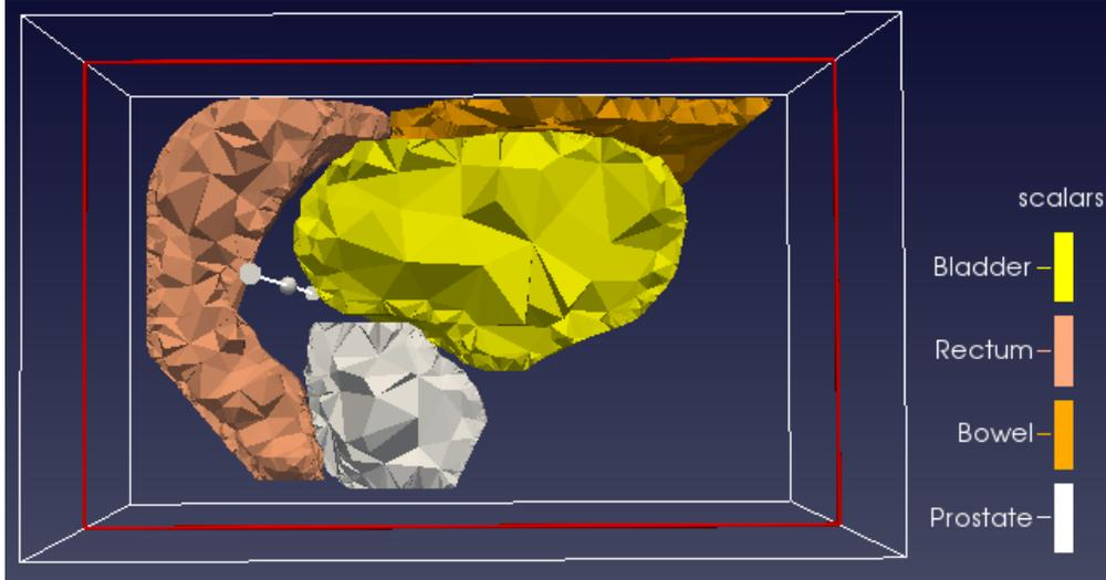
Figure 3. Cut showing the refinement achieved based on tetra volume and shape (1.7 M tetrahedra total). Note the grading of mesh size from fine at the boundaries to coarse in the interior. Propagation calculations are affected only by correct assignment of material to region. Fluence resolution depends on the size and shape of the elements over which absorption is integrated. Particularly in the bladder, the fluence in the interior is not particularly interesting.
