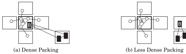
Fig. 3. Packing density and wire length example.
