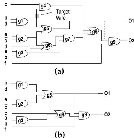
Figure 1: Optimization through rewiring
