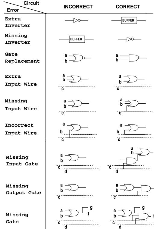
Figure 2: Design error types
