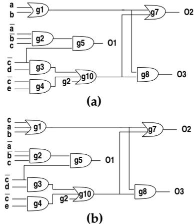
Figure 6: (a) Final Design (b) An Erroneous Design
