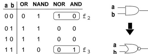
Figure 7: Fault modeling of a gate replacement error
